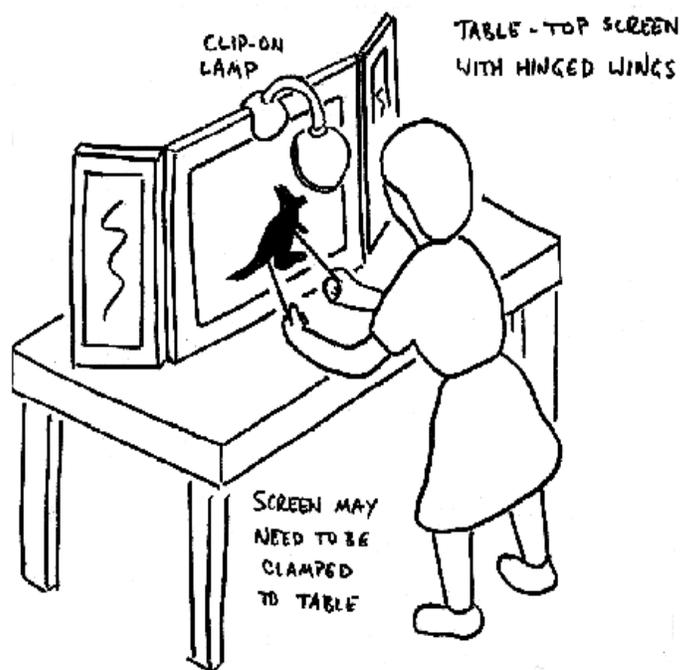
The ends of the little wire joints sometimes catch on a cloth screen but a piece of clear sticky tape over the joint on the screen side avoids this. If you find that the noise the puppets make as they move on a stretched fabric screen is annoying, you could consider putting a layer of thin clear plastic across it.
