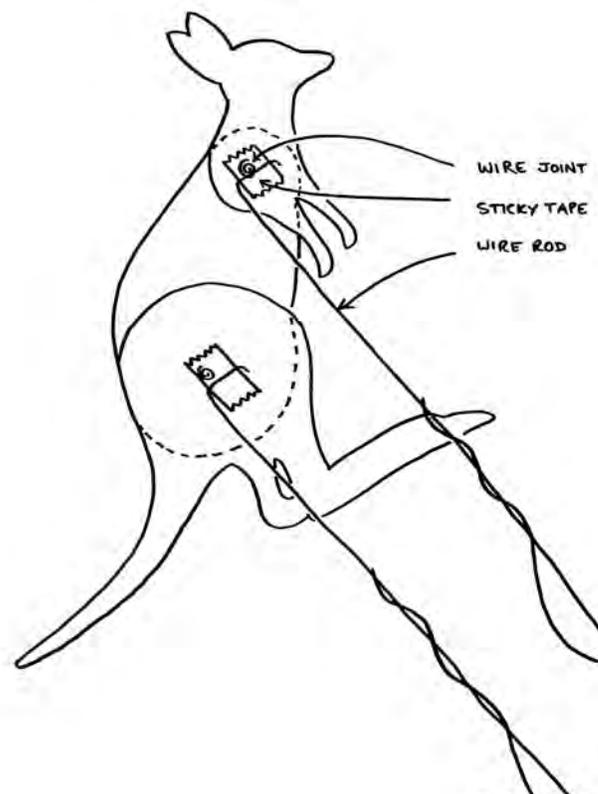
you hold one rod still with one hand, you should be able to rotate the other rod so that only the piece it is fixed to moves. If you move the rod instead of simply twisting it you can begin moving the middle part as well. If you now try moving and twisting both rods together the figure will become quite animated.
